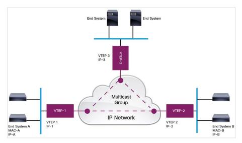
Figure 4. VXLAN Multicast Group in Transport Network
