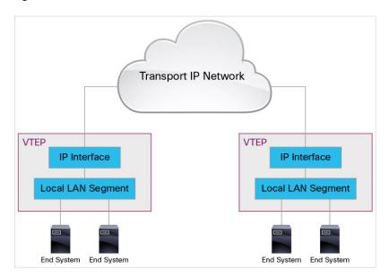
The VXLAN segments are independent of the underlying network topology; conversely, the underlying IP network between VTEPs is independent of the VXLAN overlay. It routes the encapsulated packets based on the outer IP address header, which has the initiating VTEP as the source IP address and the terminating VTEP as the destination IP address.
