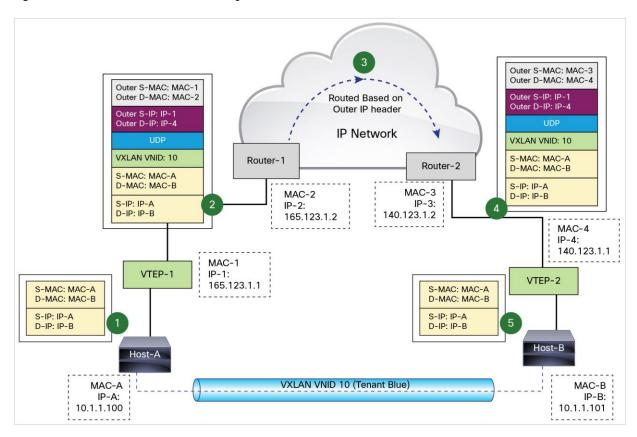
In Figure 3, Host-A and Host-B in VXLAN segment 10 communicate with each other through the VXLAN tunnel between VTEP-1 and VTEP-2. This example assumes that address learning has been done on both sides, and corresponding MAC-to-VTEP mappings exist on both VTEPs.
