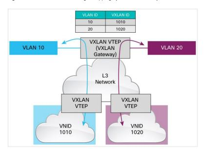
Figure 6. VXLAN-to-VLAN Logic Mapping by VXLAN Gateway
